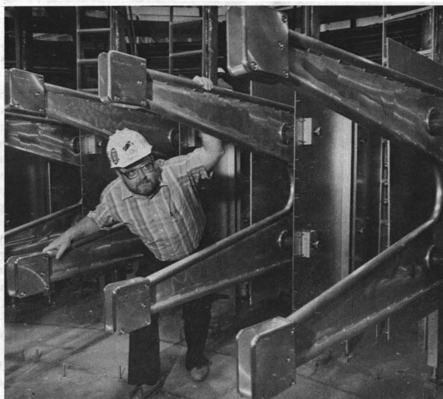
A FOREST of triplate transmission lines — and Larry Choate (1233).
